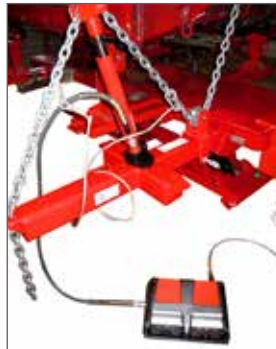
Down pull with pulley
