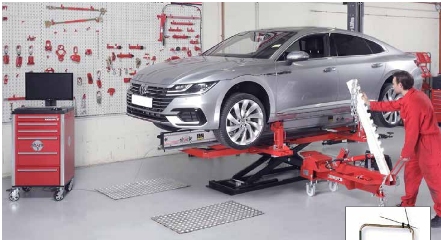
Measuring of high test point (Mc Pherson)
