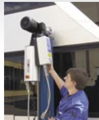
Mobile power supply unit, no master column.
